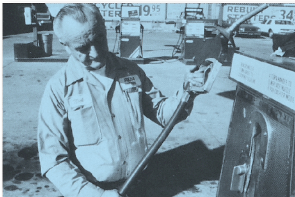
Inspect hose cover for cracks or cuts.
