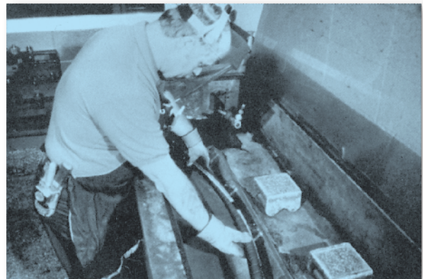
Hydrostatic hose testing.
