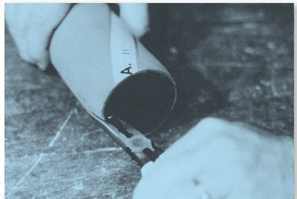
Pinching the staple into the tube wall.
