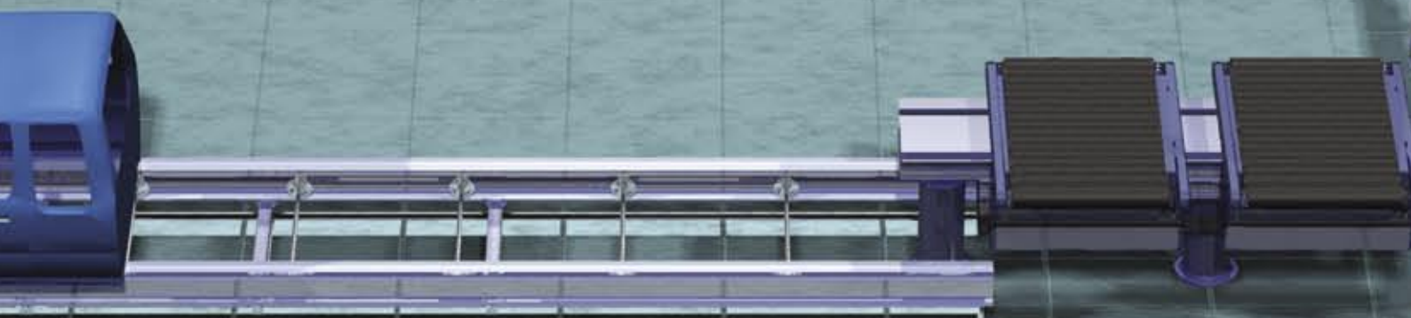
Diverter and sorter drive PowerGrip® GT3 and TransMotion™ belts
